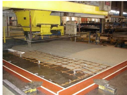
**Figure 13: The proposed mixes are used in the manufacturing process and cast using bins.**
