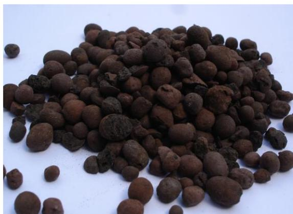
Figure 1: 4/8 fraction Argex aggregates
