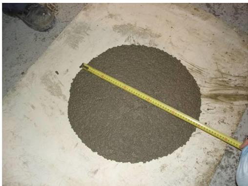
**Figure 13: It is important to monitor the properties of fresh SCC (in this case, flowability or "slump flow").**
