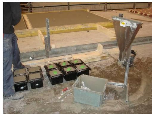
**Figure 14: Preparation of cubes, in order to monitor compressive strength and dry density**
