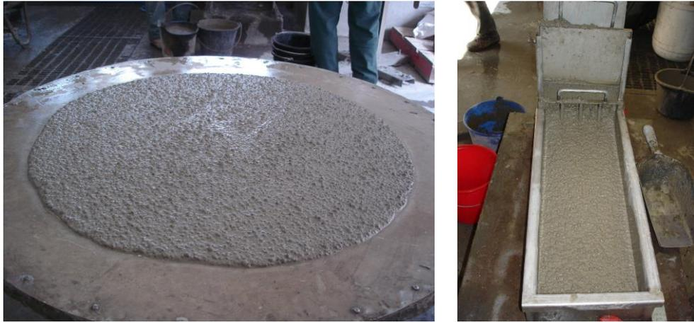
**Figure 8: Spreadability test (left) and L-box ratio (right)**
