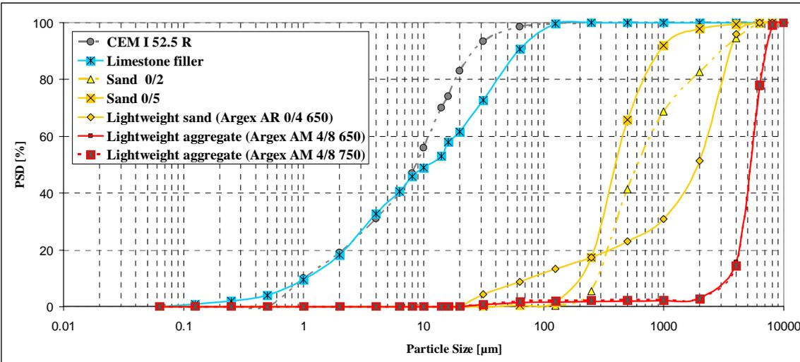
Figure 1: Particle size distributions (PSD) of the basic materials used in the testing program
