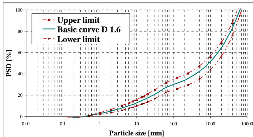
Figure 5: Basic curve for the optimisation of D-class 1.6 mixtures. The curve was established based on an empirical correction of the modified A&A-model.
