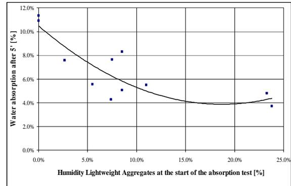
Figure 4: Water absorption of the aggregate (AM 4/8-650) after 5', starting from a specific humidity.
