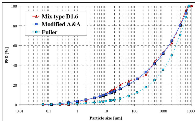
Figure 2: Result of an optimisation with the modified Andreasen and Andersen model for a mixture of type D 1.6. The figure illustrates the difference between the Fuller grading and the A&A grading. This last one appears to be very suitable for SCC.
