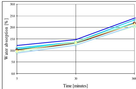
Figure 3: Water absorption of the lightweight aggregate (AM 4/8-650), starting from oven-dry condition.
