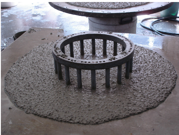
No segregation thanks to the well mix design (concrete grading etc) as the use of stabilizer.
