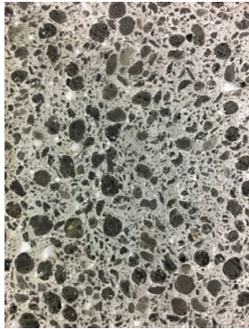
Matrix with normal coarse aggregates & Argex light sand, coarse & light sand Argex and Argex coarse aggregates & normal sand
