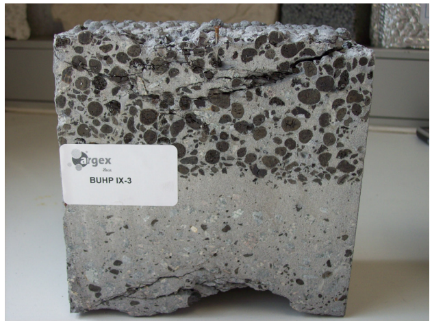
Examples of segregation of fresh concrete (bleeding) and of hard concrete.
