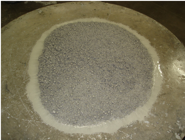
Examples of segregation of fresh concrete (bleeding) and of hard concrete.
