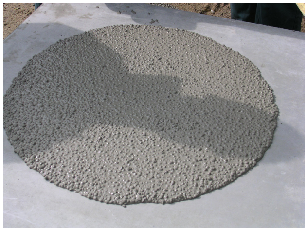
No segregation thanks to the well mix design (concrete grading etc) as the use of stabilizer.
