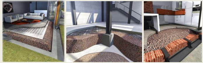
Figure 2: Examples of lightweight expanded clay aggregate in thermal insulation applications
